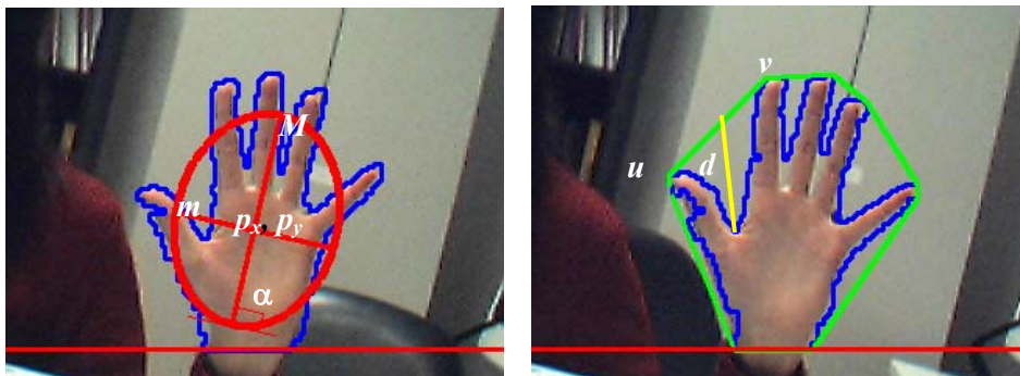
Figure 4: Extracted features for the hand gesture recognition. In the right image, u_i and v_i indicate the start and the end points of the i th-convexity defect, the depth, d_i , is the distance from the farthestmost point of the convexity defect to the convex hull segment.
